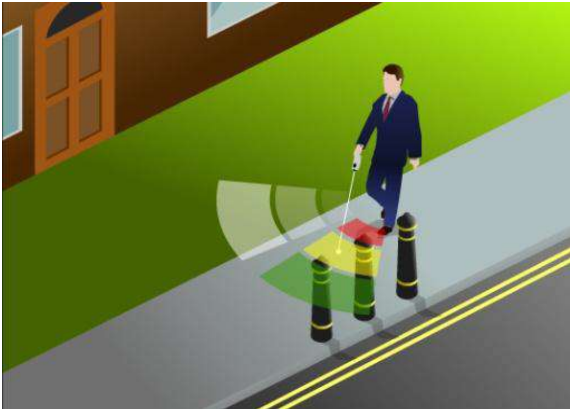
Image 5 – Obstacle detection by using Buzzer with various patterns
